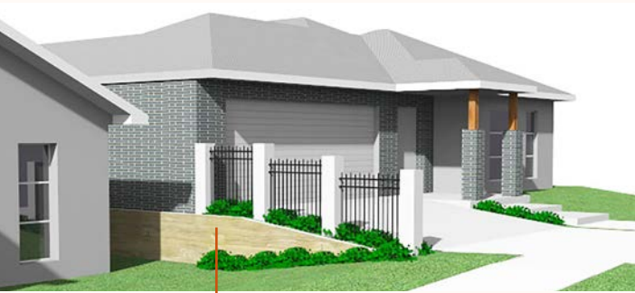
Side retaining walls forward to the house
