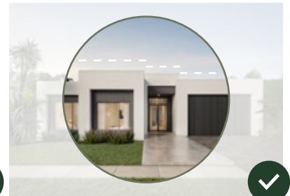
Example of suitable parapet roof
