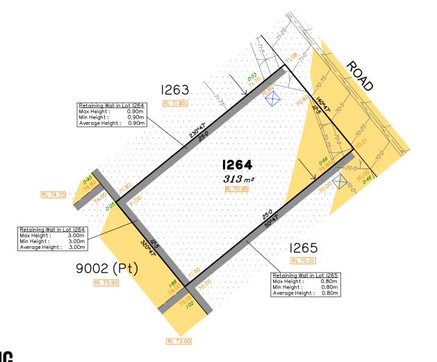
LEGEND Area of Cut Area of Fill Design Contours Depth of Fill Top of Batter Toe of Batter Retaining Wall Preferred Earthworks Pad Level Finished Surface Design Level Optional Built to Boundary Wall 300mm x 300mm Subsurface Drainage Pit
