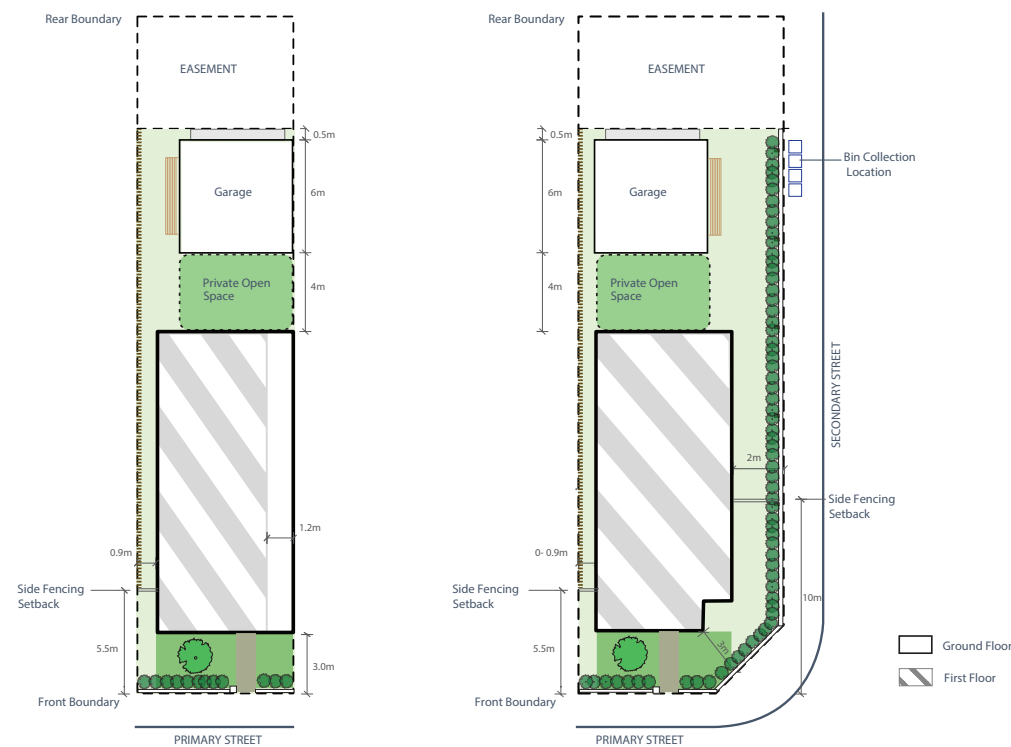
Figure 5: Front fencing & landscaping on a standard lot
