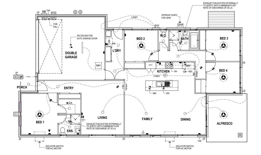
POSITION OF ELECTRICAL POINTS SUBJECT TO CONSTRUCTION CONSTRAINTS
