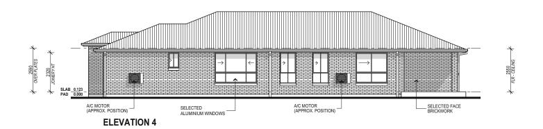
PROVIDE FULL HT. MASONRY ARTICULATION AS PER ENGINEERS SOILTEST REPORT
