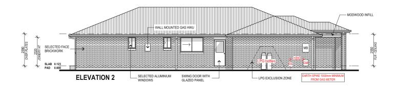
PROVIDE FULL HT. MASONRY ARTICULATION AS PER ENGINEERS SOILTEST REPORT
