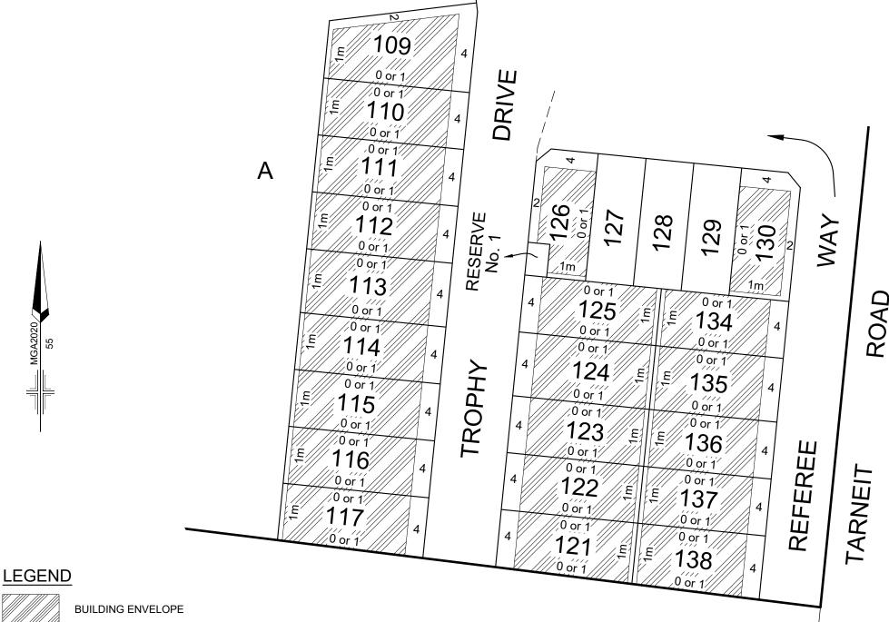
NOTE: FOR SETBACKS SHOWN "0 or 1", ONLY ONE SIDE BOUNDARY MAY BE BUILT TO WHICH ACCORDS WITH THE CROSSOVER LOCATION
