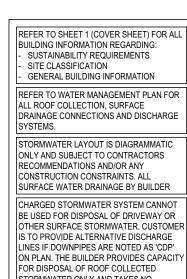
CHARGED STORMWATER SYSTEM CANNOT BE USED FOR DISPOSAL OF DRIVEWAY OR OTHER SURFACE STORMWATER. CUSTOME IS TO PROVIDE ALTERNATIVE DISCHARGE LINES IF DOWNPIPES ARE NOTED AS 'COP' ON PLAN. THE BUILDER PROVIDES CAPACIT FOR DISPOSAL OF ROOF COLLECTED STORMWATER ONLY AND TAKES NO RESPONSIBILITY FOR OVERFLOW OR DAMAGE TO PROPERTY IF CUSTOMER ADDS ADDITIONAL DISCHARGE LOADS TO EXISTING STANDARD PROVISIONS.
