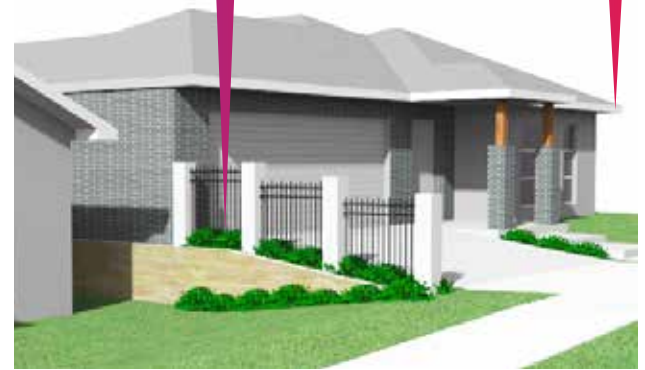
Retaining walls forward of the home must taper on side boundaries
