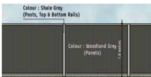
Corner fencing detail
