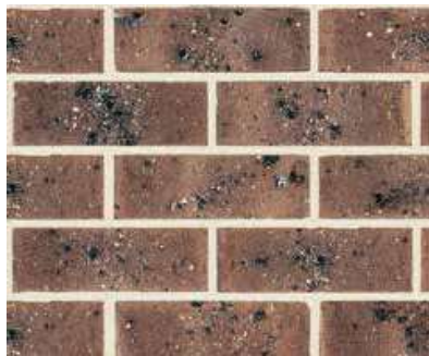
Unaccepted fritted brick example
