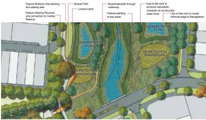
Additional sedimentation ponds will replenish and recycle community water, and support bioretention raingardens along the waterways.
